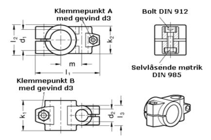
Adjustable clamp lever for d3 = GN 911-M 8-32 have to be ordred separately Adjustable clamp lever for d4 = GN 911-M 6-25 have to be ordred separately d1 = 25 d2 = 12 d3 = M 8 d4 = M 6
